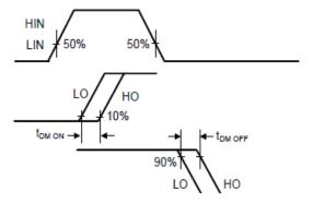
Figure 1. Switching Time Waveform Definitions
