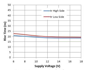
Figure 8. Rise Time vs. Supply Voltage
