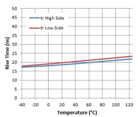
Figure 9. Rise Time vs. Temperature
