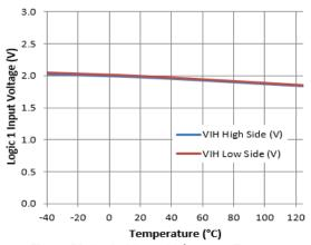
Figure 21. Logic 1 Input Voltage vs. Temperature
