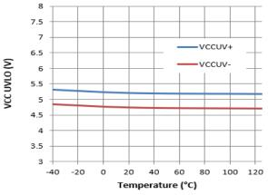
Figure 24. VCC UVLO vs. Temperature
