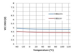
Figure 25. VBS UVLO vs. Temperature
