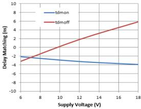
Figure 14. Delay Matching vs. Supply Voltage
