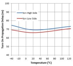
Figure 5. Turn-on Propagation Delay vs. Temperature
