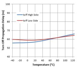
Figure 7. Turn-off Propagation Delay vs. Temperature
