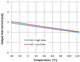
Figure 19. Output Sink Current vs. Temperature
