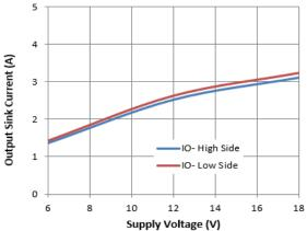
Figure 18. Output Sink Current vs. Supply Voltage
