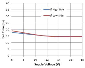
Figure 10. Fall Time vs. Supply Voltage
