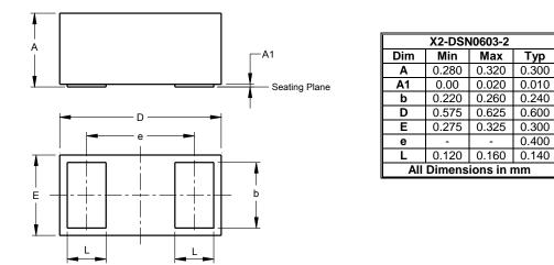
Note 7. Device side walls are electrically active bare silicon. Avoid contact of solder or flux on the side walls during the PCB assembly process.
