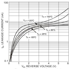
Figure 4 Typical Reverse Characteristics
