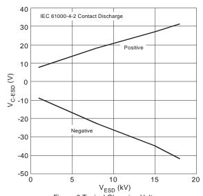
Figure 6 Typical Clamping Voltage vs. Contact Discharge Voltage
