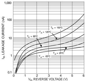
Figure 4. Typical Reverse Characteristics
