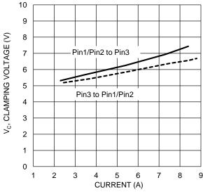
Figure 6 Clamping Voltage Characteristic (t<sub>P</sub> = 8/20µs)
