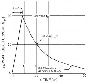
Figure 1 Typical 8×20µs Puls Waveform
