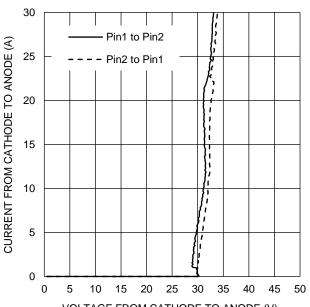
VOLTAGE FROM CATHODE TO ANODE (V) Figure 5 TLP Curve ( $t_P = 100ns$ )
