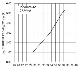
$\rm V_{\rm C}$  FROM  $\rm I_{\rm O}$  TO  $\rm V_{\rm SS}$  (V) Figure 4 Clamping Voltage Characteristic
