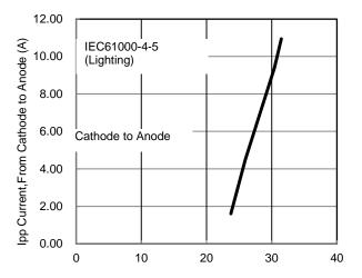
Vc FROM Cathode to Anode (V) Figure 5 Clamping Voltage Characteristic
