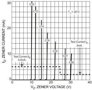
Figure 4 Typical Zener Breakdown Characteristic
