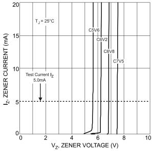
Figure 3 Typical Zener Breakdown Characteristic
