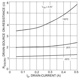
Fig. 7 Drain-Source On-Resistance vs. Drain-Current
