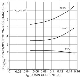
Fig. 5 Drain-Source On-Resistance vs. Drain-Current
