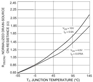
Fig. 3 Drain-Source On-Resistance vs. Junction Temperature
