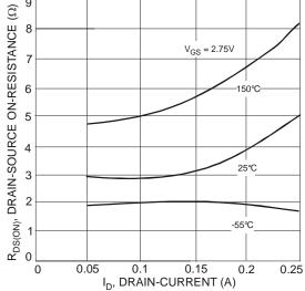
Fig. 6 Drain-Source On-Resistance vs. Drain-Current
