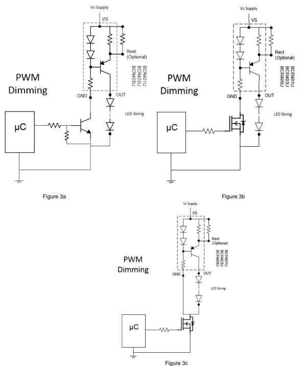
Figure 3a, 3b & 3c Application Circuits for LED Driver with PWM Dimming Functionality
