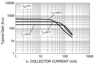
Figure 4. h<sub>FE</sub> v I<sub>C</sub>
