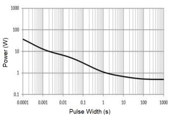
Fig.4 Power vs Pulse Width
