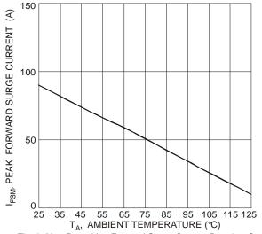
Fig. 8 Non-Repetitive Forward Surge Current Derating Curve
