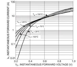
Fig. 1 Typical Forward Characteristics - B320AQ thru B340AQ
