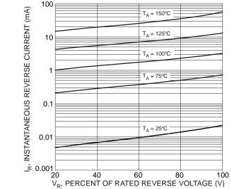
Fig. 3 Typical Reverse Characteristics, B320AQ thru B340AQ
