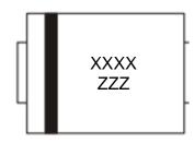
XXXX : Assembly Tracing code ZZZ : Product Type Marking code Bar Denotes Cathode Side
