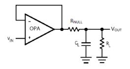
Figure 3. Capacitive Load with RNULL
