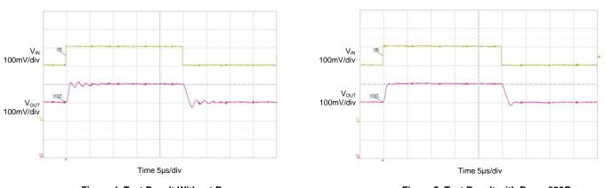
Figure 4. Test Result Without R<sub>NULL</sub>
