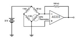
Figure 8. Bridge Circuit Amplification
