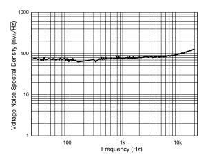
Figure 2. Input Voltage Noise in Zero-Drift Amplifier
