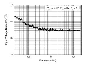
Figure 1. Input Voltage Noise in Conventional Amplifier
