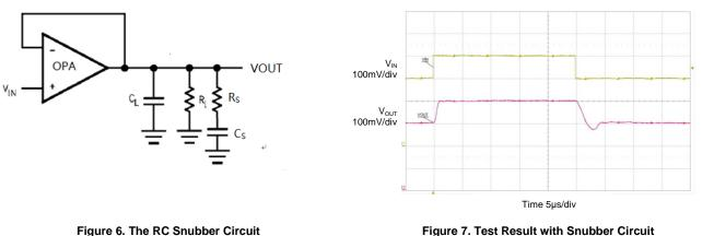
Figure 7. Test Result with Snubber Circuit
