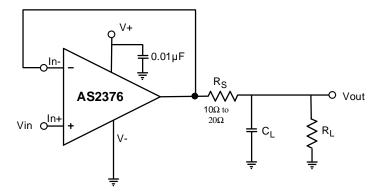
Circuit for Driving Large Capacitive Loads
