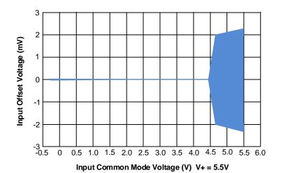
Offset Voltage over Common Mode Voltage Range
