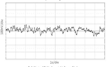
0.1-Hz to 10-Hz Input Voltage Noise
