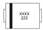
XXXX : Assembly Tracing Code ZZZ : Product Type Marking Code Bar Denotes Cathode Side
