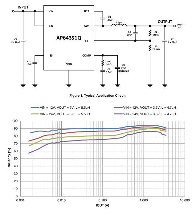
Figure 2. Efficiency vs. Output Current
