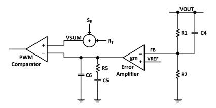
Figure 26. Type II Compensator
