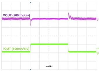
Figure 16. Load Transient, IOUT = 50mA to 500mA to 50mA
