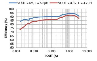
Figure 4. Efficiency vs. Output Current, VIN = 12V
