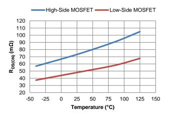
Figure 9. Power MOSFET RDS(ON) vs. Temperature
