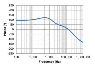
Figure 30. Closed-Loop Phase Margin
