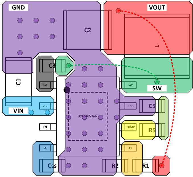
Figure 31. Recommended PCB Layout
