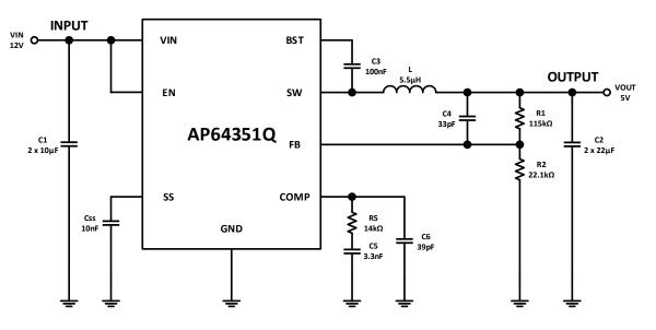
Figure 28. Example Circuit with Calculated Component Values for Loop Compensation
