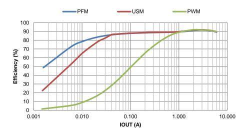
Figure 3. Efficiency vs. Output Current, VIN = 12V, VOUT = 3.3V, L = 1.2µH, fsw = 800kHz
