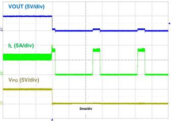
Figure 11. Output Short Protection, IOUT = 6A
