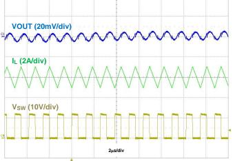
Figure 40. Output Voltage Ripple, IOUT = 50mA
