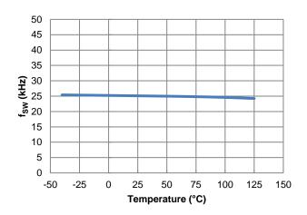
Figure 27. f<sub>SW</sub> vs. Temperature, IOUT = 0A
