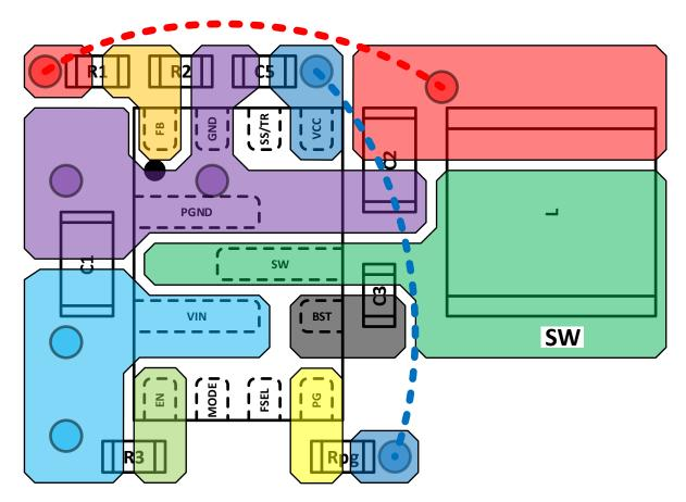
Figure 53. Recommended PCB Layout
