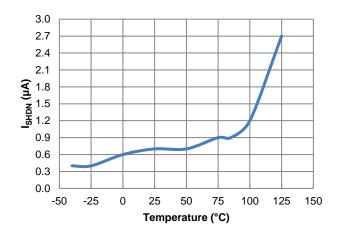
Figure 7. ISHDN vs. Temperature
