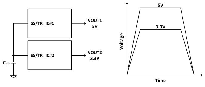
Figure 45. Ratiometric Tracking Configuration
