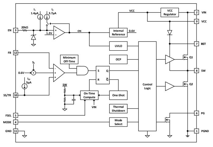
Figure 4. Functional Block Diagram
