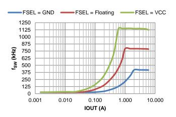
Figure 28. fsw vs. Load
