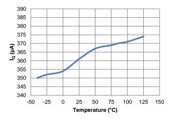
Figure 16. IQ vs. Temperature
