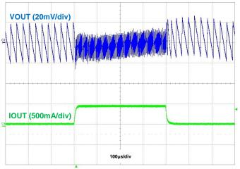
Figure 20. Load Transient, IOUT = 50mA to 500mA to 50mA
