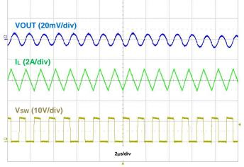
Figure 18. Output Voltage Ripple, IOUT = 50mA
