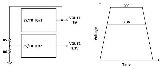
Figure 47. Coincidental Tracking Configuration
