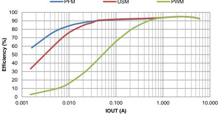
Figure 2. Efficiency vs. Output Current, VIN = 12V, VOUT = 5V, L =  $1.5\mu$ H, fsw = 800kHz
