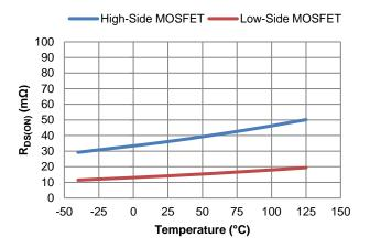
Figure 5. Power MOSFET RDS(ON) vs. Temperature
