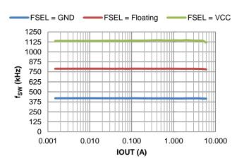
Figure 39. fsw vs. Load
