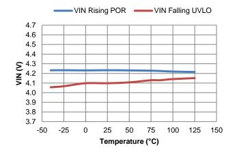
Figure 8. VIN Power-On Reset and UVLO vs. Temperature
