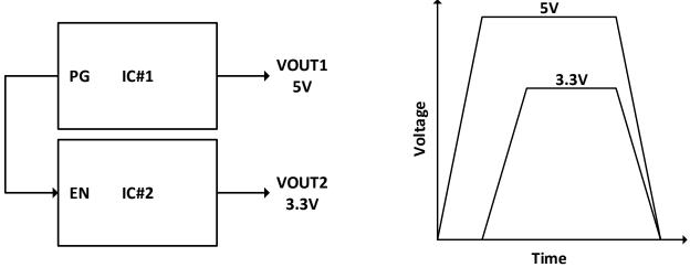
Figure 49. Output Sequencing Configuration
