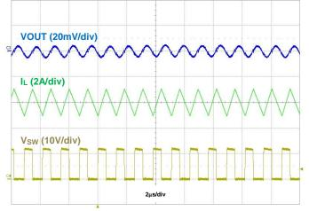
Figure 29. Output Voltage Ripple, IOUT = 50mA
