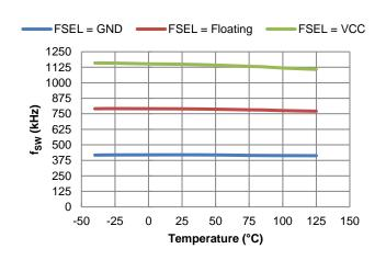
Figure 38. fsw vs. Temperature, IOUT = 0A
