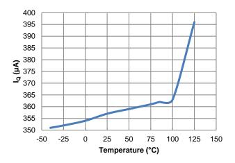
Figure 37. IQ vs. Temperature
