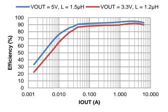
Figure 23. Efficiency vs. Output Current, VIN = 12V
