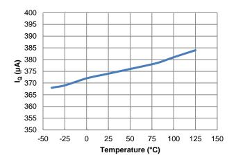
Figure 26. I<sub>Q</sub> vs. Temperature
