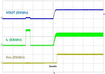
Figure 12. Output Short Recovery, IOUT = 6A
