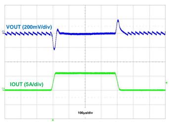
Figure 22. Load Transient, IOUT = 50mA to 6A to 50mA
