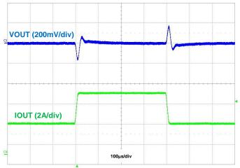
Figure 21. Load Transient, IOUT = 3A to 6A to 3A
