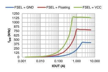
Figure 17. fsw vs. Load
