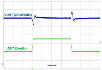
Figure 32. Load Transient, IOUT = 3A to 6A to 3A
