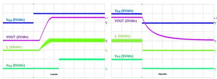
Figure 10. Startup Using EN, Showing  $V_{PG}$ , IOUT = 5A
