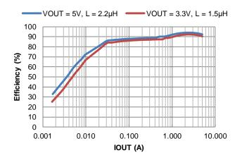
Figure 25. Efficiency vs. Output Current
