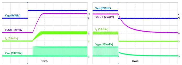
Figure 8. Startup Using EN, Showing  $V_{SW}$ , IOUT = 5A
