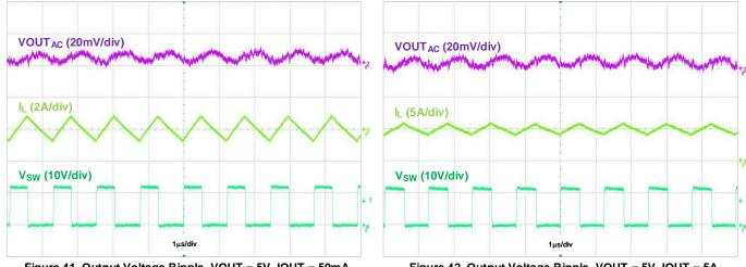
Figure 41. Output Voltage Ripple, VOUT = 5V, IOUT = 50mA
