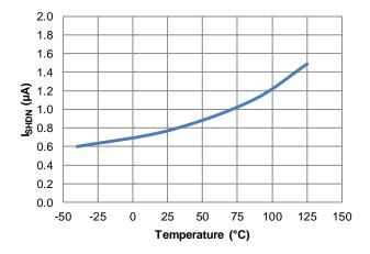
Figure 7. I<sub>SHDN</sub> vs. Temperature
