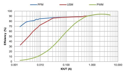
Figure 2. Efficiency vs. Output Current, VIN = 12V, VOUT = 5V, L =  $2.2\mu H$ ,  $f_{SW}$  = 800kHz
