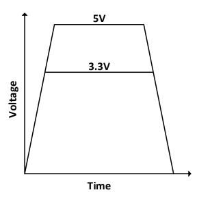
Figure 49. Coincidental Tracking Configuration
