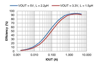
Figure 36. Efficiency vs. Output Current
