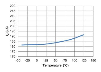
Figure 17.  $I_Q$  vs. Temperature
