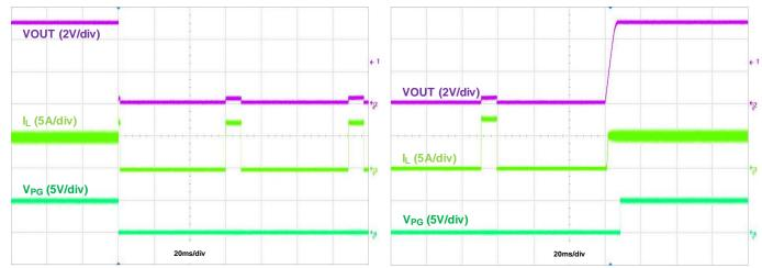
Figure 12. Output Short Protection, IOUT = 5A
