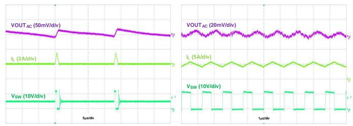
Figure 30. Output Voltage Ripple, VOUT = 5V, IOUT = 50mA
