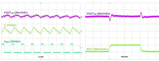
Figure 43. Output Voltage Ripple, VOUT = 3.3V, IOUT = 50mA
