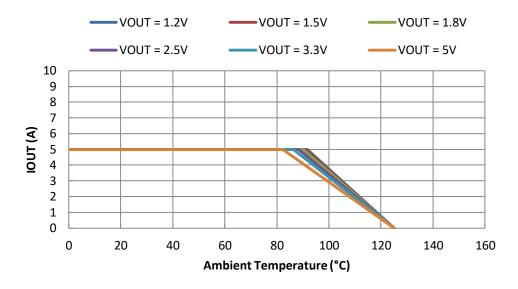
Figure 54. Output Current Derating Curve vs. Ambient Temperature, VIN = 12V, f<sub>SW</sub> = 800kHz
