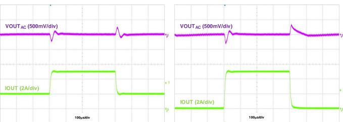
Figure 23. Load Transient, IOUT = 2A to 5A to 2A
