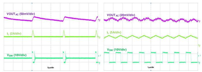
Figure 19. Output Voltage Ripple, VOUT = 5V, IOUT = 50mA
