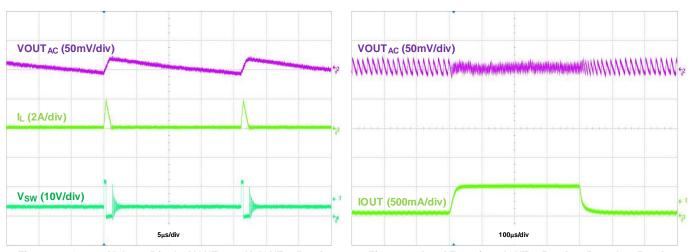
Figure 32. Output Voltage Ripple, VOUT = 3.3V, IOUT = 50mA
