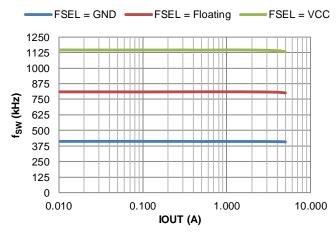
Figure 40. f<sub>SW</sub> vs. Load
