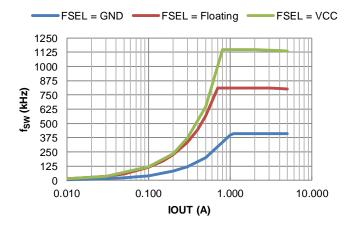
Figure 18. f<sub>SW</sub> vs. Load
