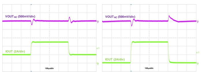
Figure 34. Load Transient, IOUT = 2A to 5A to 4A
