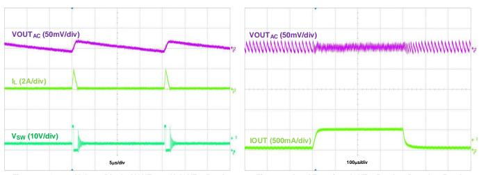
Figure 21. Output Voltage Ripple, VOUT = 3.3V, IOUT = 50mA
