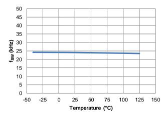
Figure 28. f<sub>SW</sub> vs. Temperature, IOUT = 0A
