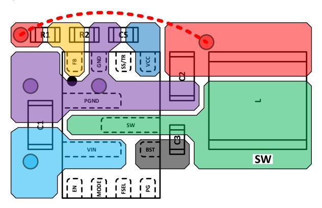
Figure 55. Recommended PCB Layout
