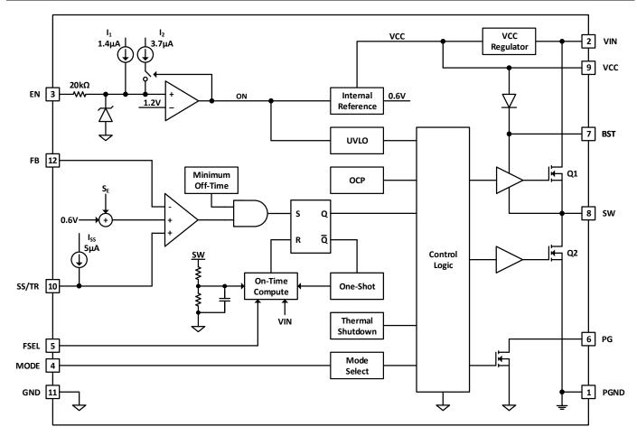
Figure 4. Functional Block Diagram
