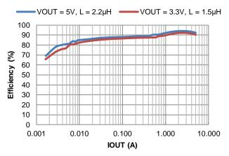
Figure 14. Efficiency vs. Output Current
