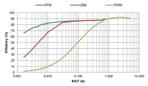
Figure 3. Efficiency vs. Output Current, VIN = 12V, VOUT = 3.3V, L = 1.5 $\mu$ H,  $f_{SW}$  = 800kHz
