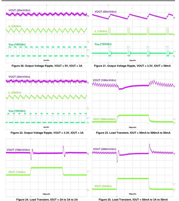
Figure 25. Load Transient, IOUT = 50mA to 3A to 50mA
