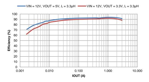
Figure 2. Efficiency vs. Output Current, AP62300/AP62300T
