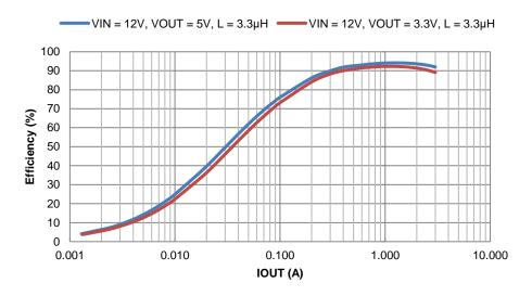
Figure 3. Efficiency vs. Output Current, AP62301
