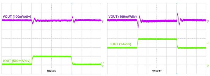
Figure 36. Load Transient, IOUT = 50mA to 500mA to 50mA
