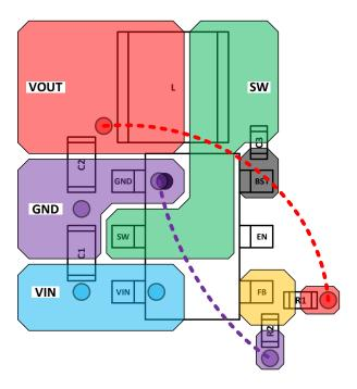
Figure 42. Recommended PCB Layout, SOT563 (Standard)
