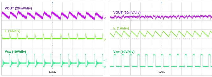
Figure 15. Output Voltage Ripple, VOUT = 3.3V, IOUT = 50mA
