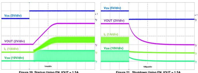
Figure 20. Startup Using EN, IOUT = 1.5A
