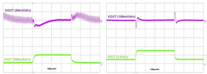
Figure 17. Load Transient, IOUT = 50mA to 500mA to 50mA
