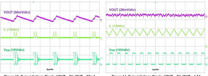
Figure 13. Output Voltage Ripple, VOUT = 5V, IOUT = 50mA
