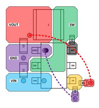
Figure 27. Recommended PCB Layout, SOT563 (Standard)
