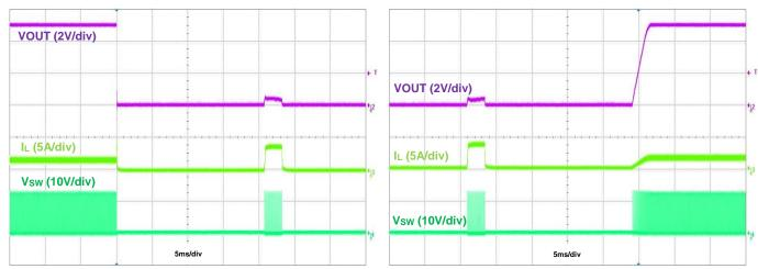
Figure 22. Output Short Protection, IOUT = 1.5A
