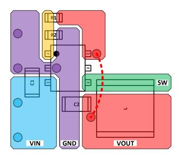
Figure 42. Recommended AP61100 PCB Layout
