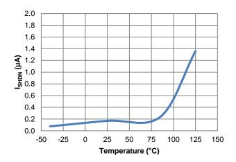
Figure 8. ISHDN vs. Temperature
