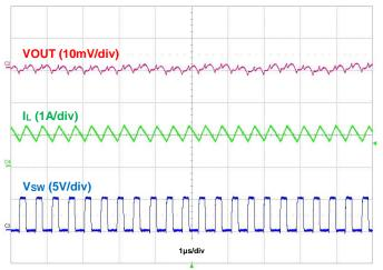
Figure 29. Output Voltage Ripple, IOUT = 1A
