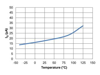
Figure 14. Io vs. Temperature
