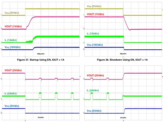
Figure 39. Output Short Protection, IOUT = 1A
