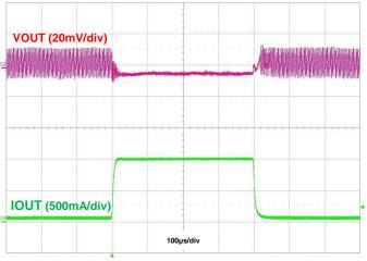
Figure 20. Load Transient, IOUT = 50mA to 1A to 50mA
