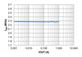
Figure 27. fsw vs. Load
