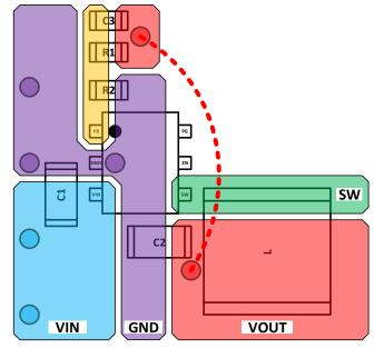
Figure 43. Recommended AP61102 PCB Layout
