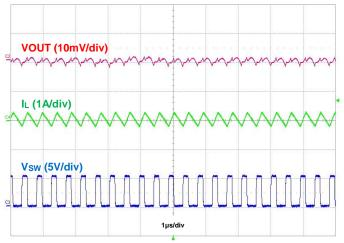
Figure 28. Output Voltage Ripple, IOUT = 50mA
