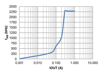
Figure 15. fsw vs. Load
