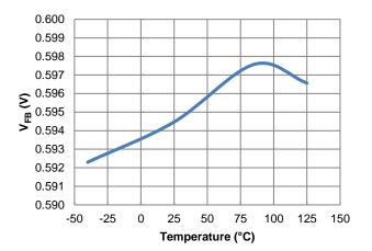
Figure 7. VFB vs. Temperature
