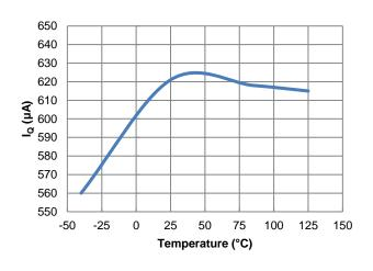
Figure 25. Io vs. Temperature
