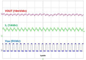
Figure 17. Output Voltage Ripple, IOUT = 1A
