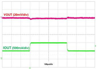
Figure 19. Load Transient, IOUT = 500mA to 1A to 500mA
