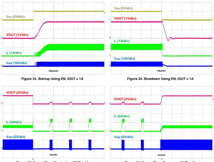
Figure 35. Output Short Protection, IOUT = 1A
