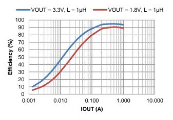
Figure 22. Efficiency vs. Output Current, VIN = 5V
