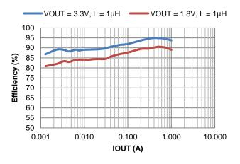
Figure 11. Efficiency vs. Output Current, VIN = 5V
