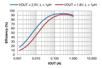
Figure 21. Efficiency vs. Output Current, VIN = 3.3V
