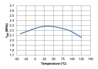
Figure 26. fsw vs. Temperature, IOUT = 0A
