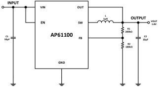
Figure 1. Typical AP61100 Application Circuit
