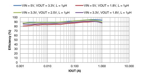
Figure 3. PFM Efficiency vs. Output Current
