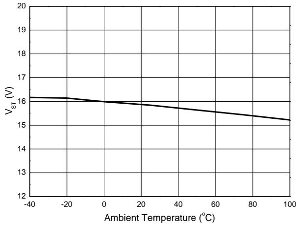
**V<sub>UVLO</sub> vs. Ambient Temperature**
