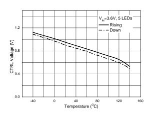
**OVP Voltage vs. Temperature**
