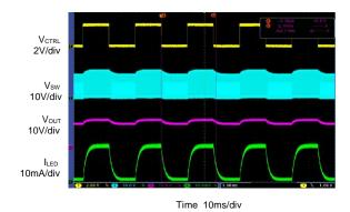
PWM Dimming  $(V_{\text{IN}}=3.6V,\,V_{\text{PWM}}=2.5V,\,f_{\text{PWM}}=100k\text{Hz},\\ \text{Duty}=50\%,\,5~\text{LEDs})$
