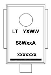
LT = Manufacturer's Code Marking S8WxxA = Product Type Marking Code YXWW = Date Code Marking Y = Last Digit of Year (ex: 3 = 2023) X = Manufacturer's Internal Code WW = Week Code (01 to 53) xxxxxxx = Assembly Tracking Code Cathode Bar
