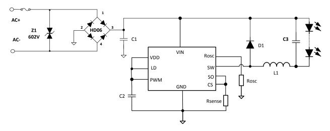
Figure 1 Typical Application Circuit (without PFC)
