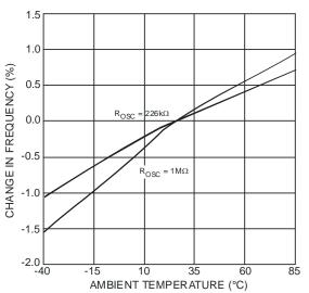
Change in Oscillation Frequency vs. Ambient Temperature
