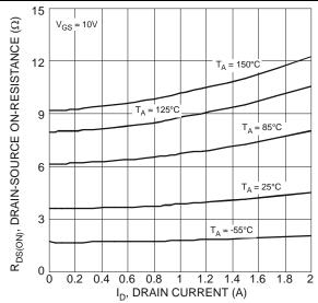
Typical On-Resistance vs. Drain Current and Temperature
