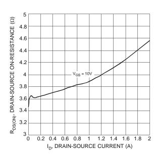
Typical On-Resistance vs. Drain Current and Gate Voltage
