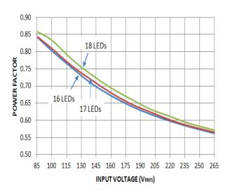
180mA LED Driver Power Factor vs. Input Voltage
