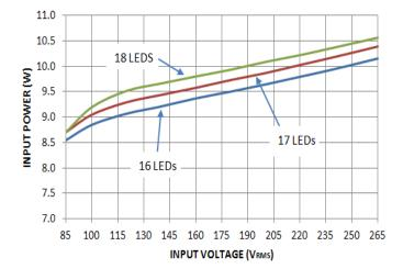
180mA LED Driver Input Power Dissipation vs. Input Voltage
