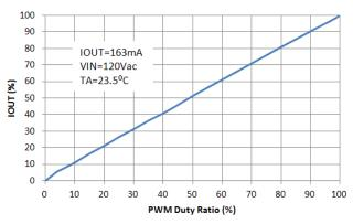
IOUT vs. PWM Dimming Control at 1KHz
