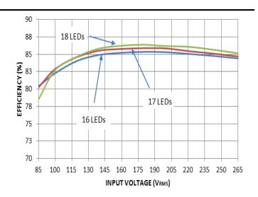
180mA LED Driver Efficiency vs. Input Voltage
