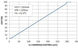
IOUT vs. V<sub>LD</sub> Dimming Control
