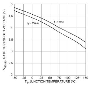
Gate Threshold Variation vs. Ambient Temperature
