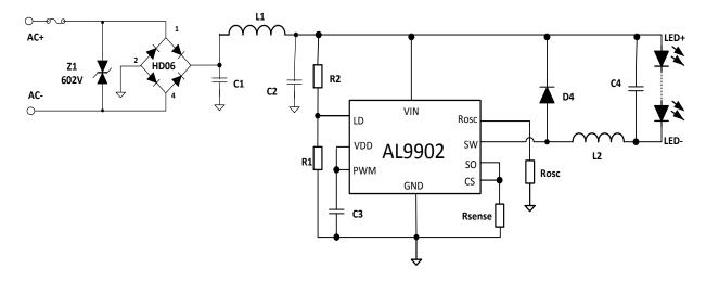
Figure 2 Typical Application Circuit with Simple PFC
