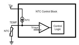
Figure 6. Temp Detection Diagram
