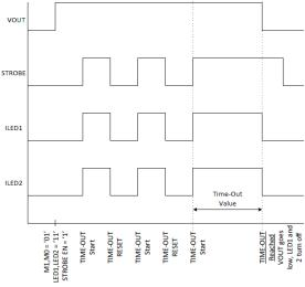
Figure 4. IR Mode Timeout 12 of 25 www.diodes.com
