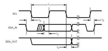
Figure 1. I<sup>2</sup>C-Compatible Interface Specifications
