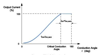
Figure 2. TRIAC Dimming Curve
