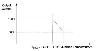
Figure 1. Thermal Foldback Waveform
