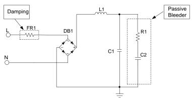
Figure 3. LED Driver Schematic with Passive Bleeder
