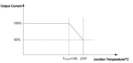
Figure 1. Thermal Foldback Waveform
