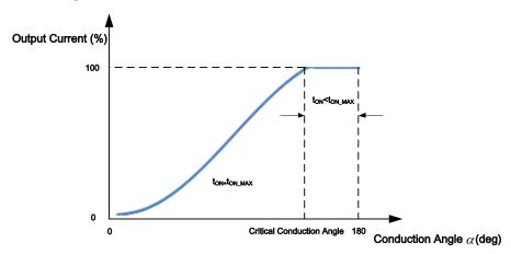
Figure 2. Dimming Curve
