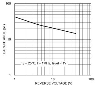
Figure 4. Typcial Junction Capacitance
