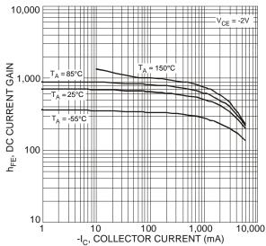
Figure 3. Typical DC Current Gain vs. Collector Current
