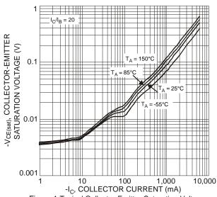
Figure 4. Typical Collector-Emitter Saturation Voltage vs. Collector Current
