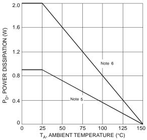
Figure 1. Power Dissipation vs. Ambient Temperature
