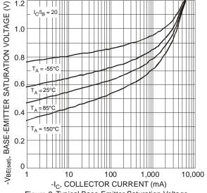
Figure 6. Typical Base-Emitter Saturation Voltage vs. Collector Current
