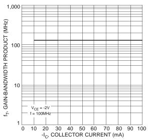
Figure 8. Typical Gain-Bandwidth Product vs. Collector Current
