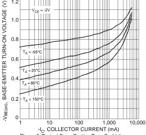
Figure 5. Typical Base-Emitter Turn-On Voltage vs. Collector Current
