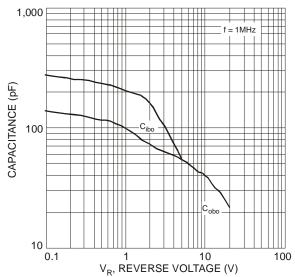
Figure 7. Typical Capacitance Characteristics
