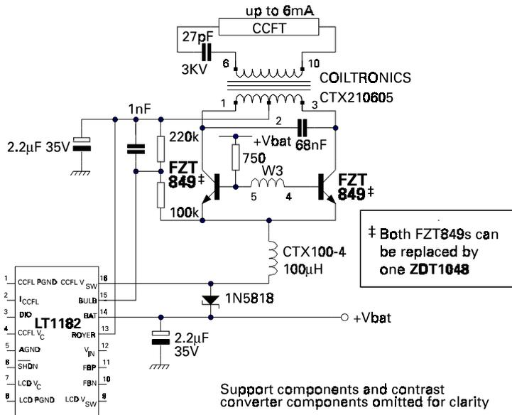
Figure 6. Linear Technology Floating Tube LCD Backlight Converter.
