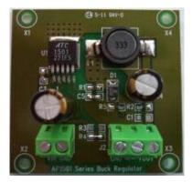
This demonstration board allows the designer to evaluate the performance of the AP1501 series buck regulator in a typical application circuit. The user needs only to supply an input voltage and a load. The demonstration board can be configured to evaluate a fixed output voltage of 3.3V, 5V, 12V, and an adjustable output version of the AP1501 series. Operation at other voltages and currents may be accomplished by proper component selection and replacement.
