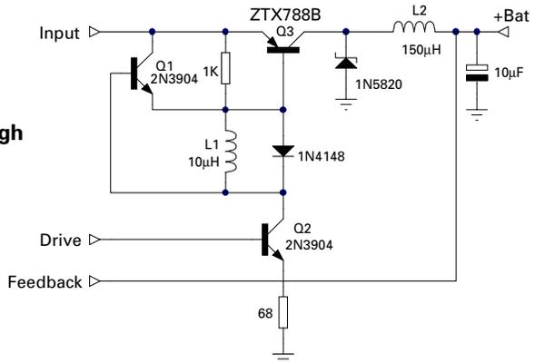
The turn-off circuit shown in Figure 1 can be used with an efficient PNP transistor as a cost effective alternative to P-Channel MOSFETs in step-down (Buck) converters.
