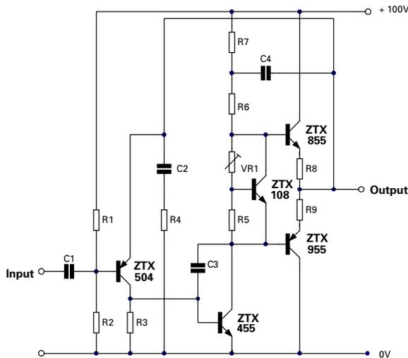
Depth/Echo sounders require high power linear amplifiers for driving the transducer. Since these amplifiers operate in pulsed mode, the average power dissipation experienced by the output transistors is low, but the value of the pulsed current can be very high. This would normally dictate that high power, large package power transistors would be required, which tends to increase the overall circuit size.
