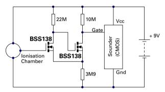
Smoke particles entering an ionising detection chamber generate signals of only a few pico-amperes. This signal must be buffered by a high input impedance amplifier, normally requiring an expensive low leakage J-FET.
