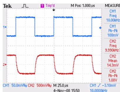
Figure 8  $G = 10$ ,  $V_{IN} = 50mV$  10kHz square wave,
