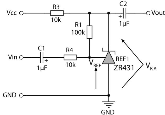
Figure 3 - Gain of 10 amplifier with unity DC gain
