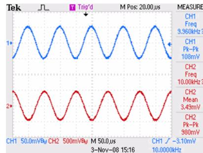
Figure 5  $G = 10$ ,  $V_{IN} = 50\text{mV}$  10kHz sine wave, load = 200R
