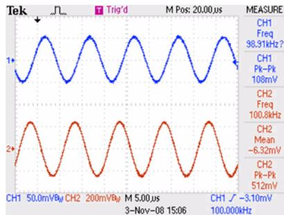
Figure 6  $G = 10$ ,  $V_{IN} = 50\text{mV}$  100kHz sine wave, load = 10k
