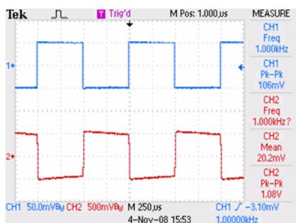
Figure 7  $G = 10$ ,  $V_{IN} = 50mV$  1kHz square wave,
