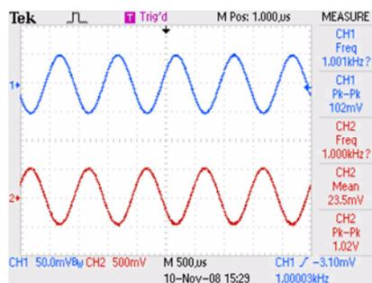
Figure 9  $G = 10$ ,  $V_{IN} = 50mV$  1kHz sine wave, load = 10k
