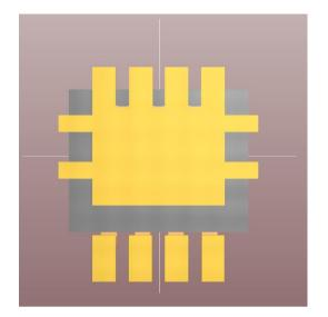
The new footprint is, by design, also compatible with PowerDI3333 as shown below:
