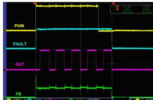
Figure 6. Dimming Minimum on Time Control
