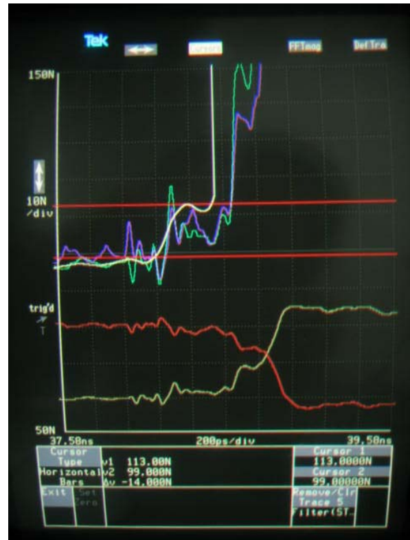
Figure 9d: TDR at CLK of Port A
