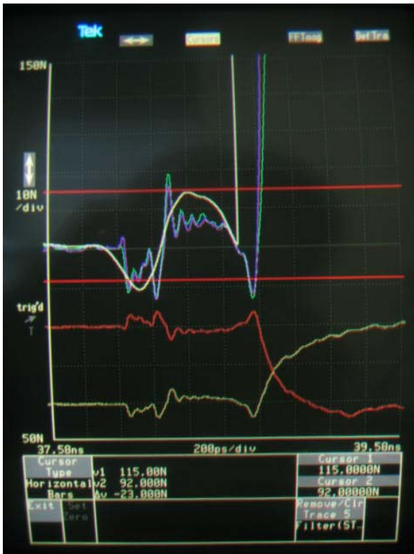
Figure 9c: TDR at D0 of Port A
