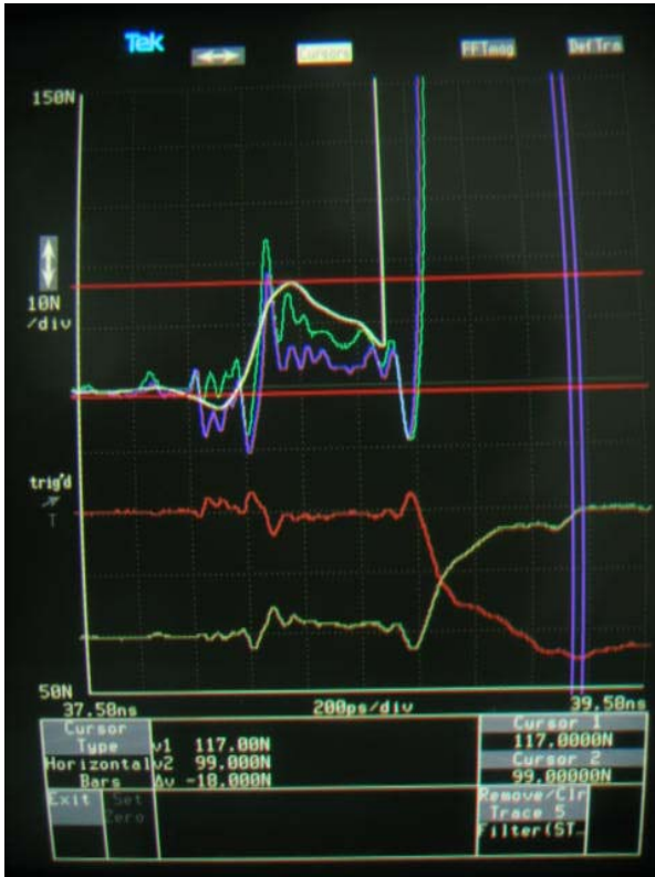
Figure 9a: TDR at D2 of Port A
