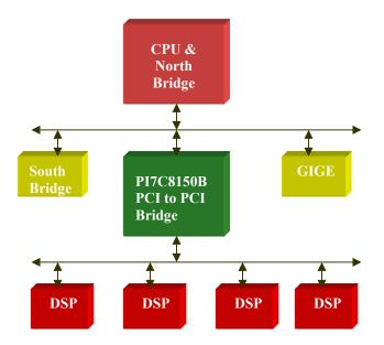
3.3 Bus isolation in order to isolate the high-speed devices from the lower speed chips.
