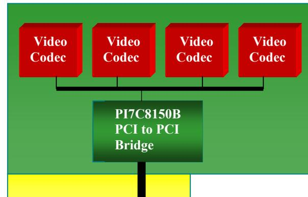
**3.3 Bus isolation in order to isolate the high-speed devices from the lower speed chips.**
