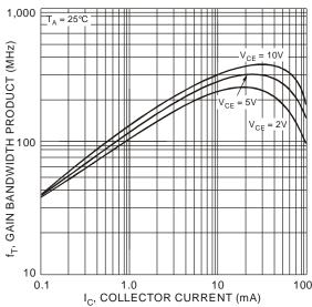
Fig. 4, Gain Bandwidth Product vs Collector Current
