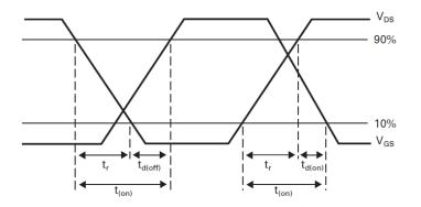
Switching time waveforms
