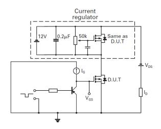
Gate charge test circuit
