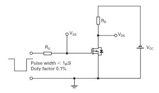
Switching time test circuit
