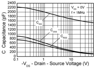
Capacitance v Drain-Source Voltage
