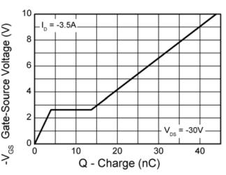
Gate-Source Voltage v Gate Charge
