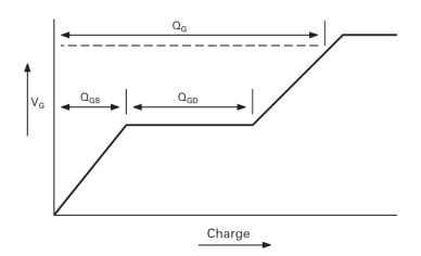
Basic gate charge waveform
