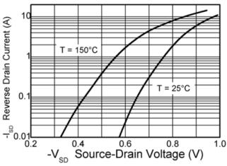
Source-Drain Diode Forward Voltage
