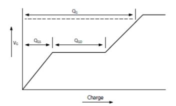
Basic gate charge waveform
