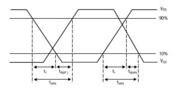
Switching time waveforms
