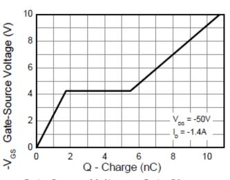
Gate-Source Voltage v Gate Charge
