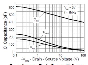
Capacitance v Drain-Source Voltage
