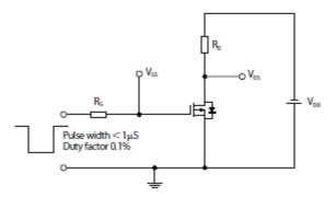
Switching time test circuit
