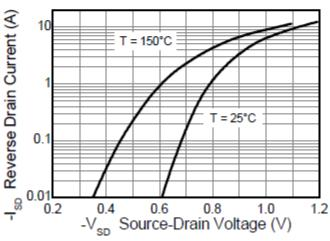
Source-Drain Diode Forward Voltage
