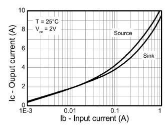
**Output current Vs Input current**
