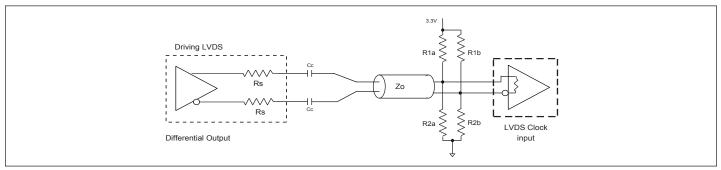
Figure 2. Differential Output Driving LVDS
