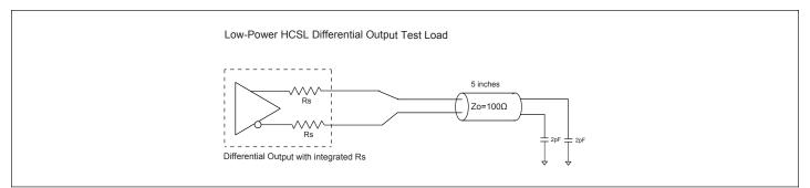
Figure 1. Low Power HCSL Test Circuit
