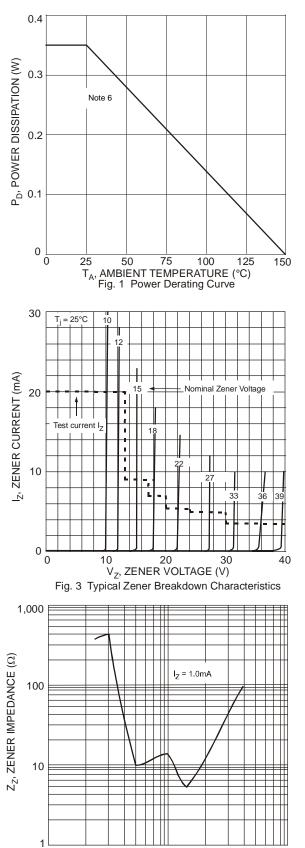
1 10 100 V<sub>Z</sub>, ZENER VOLTAGE (V) Fig. 5 Typical Zener Impedance Characteristics
